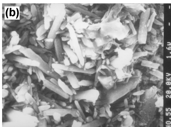
Figure 8 Interfacial morphology of the joint bonded with adhesive D: (a) sample etched in molten NaOH, (b) well developed \beta\text{-Si}_3\text{N}_4 grains in the joint. Joining condition: joining temperature, 1600 °C; holding time, 30 min; joining pressure, 5 MPa.
